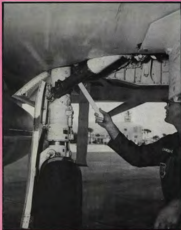
Landing gear jury struts are big and heavy.
